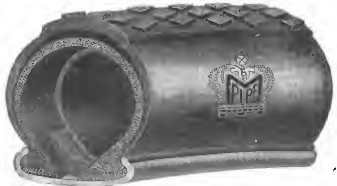
NEW CHECKERED TREAD OF EMPIRE NON-SKID TIRE
